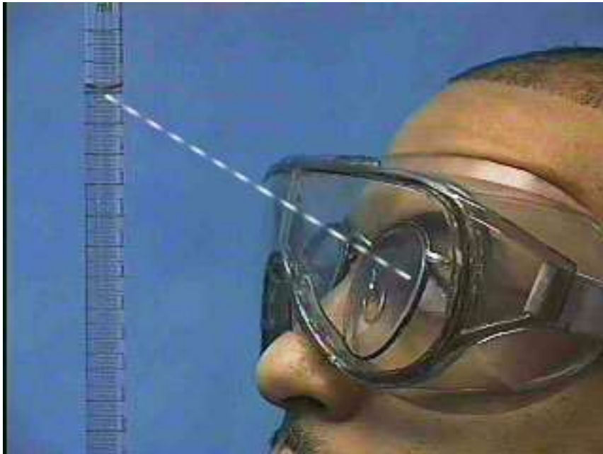
Incorrect: viewing the meniscus from an angle
